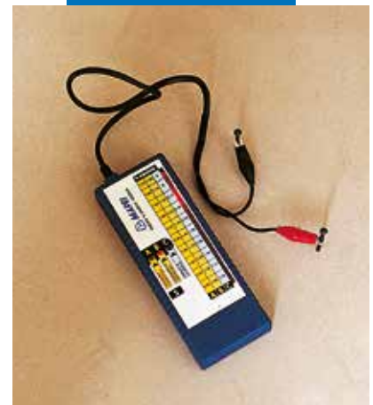
Electronic hygrometer for measuring the moisture level of a Mapecem screed
