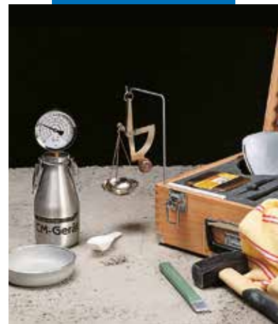
Carbide hygrometer for measuring the moisture level of a Mapecem screed
