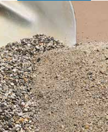
Aggregates for Mapecem: gravel from 4 to 8 mm and sand from 0 to 4 mm
