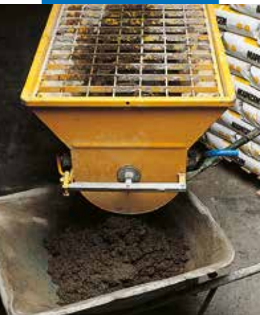
Mixing Mapecem in a mini-batcher
